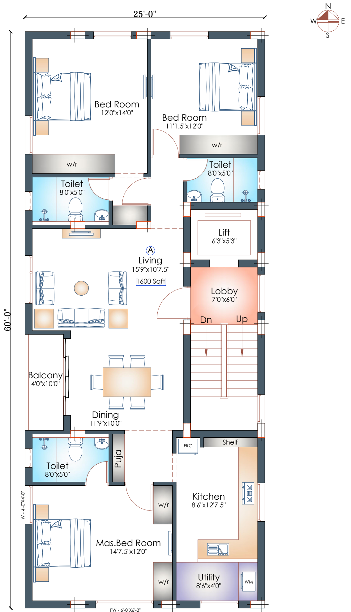
Typical Floor Plan (1st, 2nd, 3rd, 4th & 5th floor)
